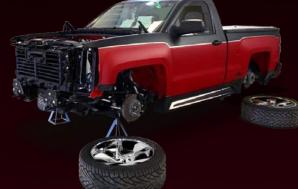
The Silverado Street Series Front Spoiler, Side Rocker Panels and Rear Skirt are inspired in the classic lowered trucks, while improving aerodynamics by redirecting the air toward the ground and away from the truck's underbody.
