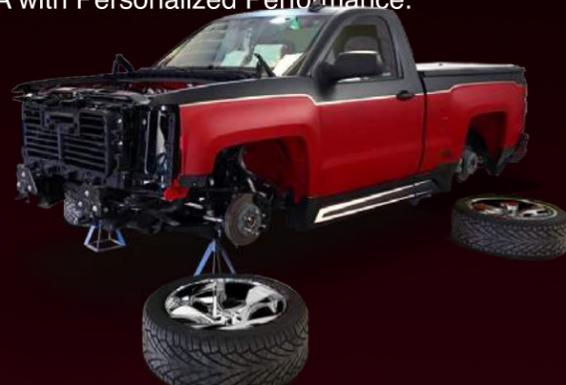
The Silverado Street Series Front Spoiler, Side Rocker Panels and Rear Skirt are inspired in the classic lowered trucks, while improving aerodynamics by redirecting the air toward the ground and away from the truck's underbody. The Silverado "Plug and Play" Styling Kit is manufactured only with the best high performance Huntsman Elastomeric Polyurethane polymers for great Flexibility and Strength, superb Surface Quality, Perfect Fit to the body and Long-Lasting Durability.
